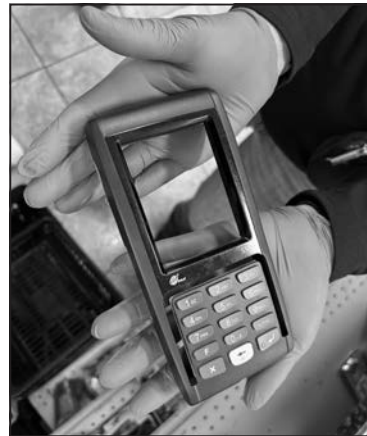
This skimming device covers the entire faceplate of a card terminal.
