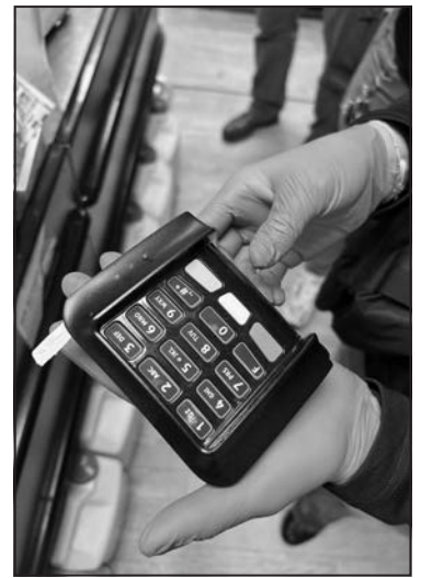
An example of one of the POS skimming devices recovered during the outreach operation.
